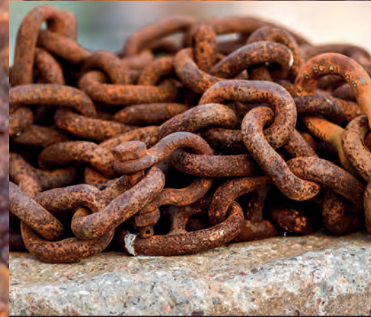
Rusty wrought iron chains at x40 zoom
